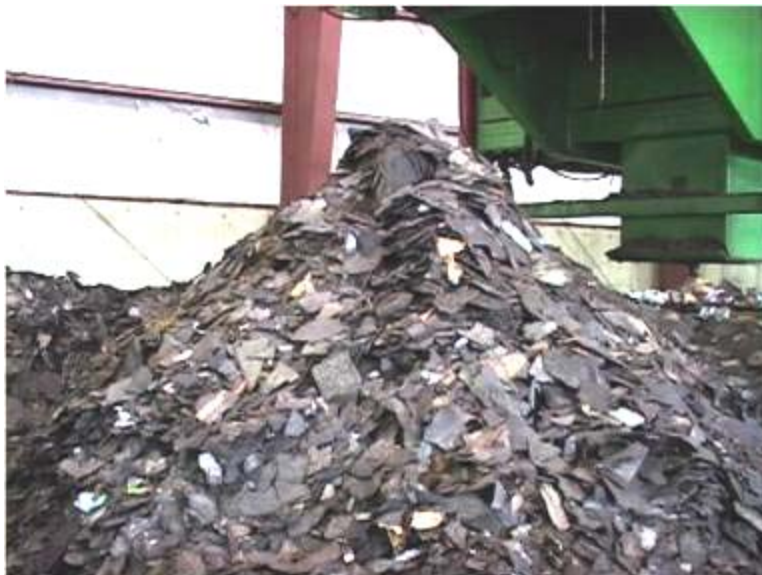
Picture 9 - Clean, Residential Tear-Off Shingles at End of Sort Line Clean, sorted shingles ready for grinding.
